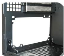
Bottom mounting PSU position supports two orientations
