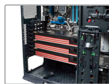
8 tool-less expansion slots
