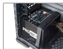
Velcro cable tie for PSU securing
